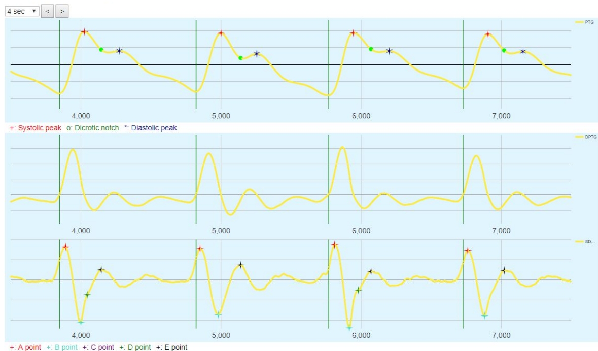
Fig. 1. -the original pulse wave, then the first and second derivative of the curve below each other
